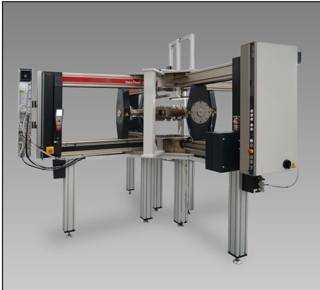
Horizontally oriented cruciform testing machine
