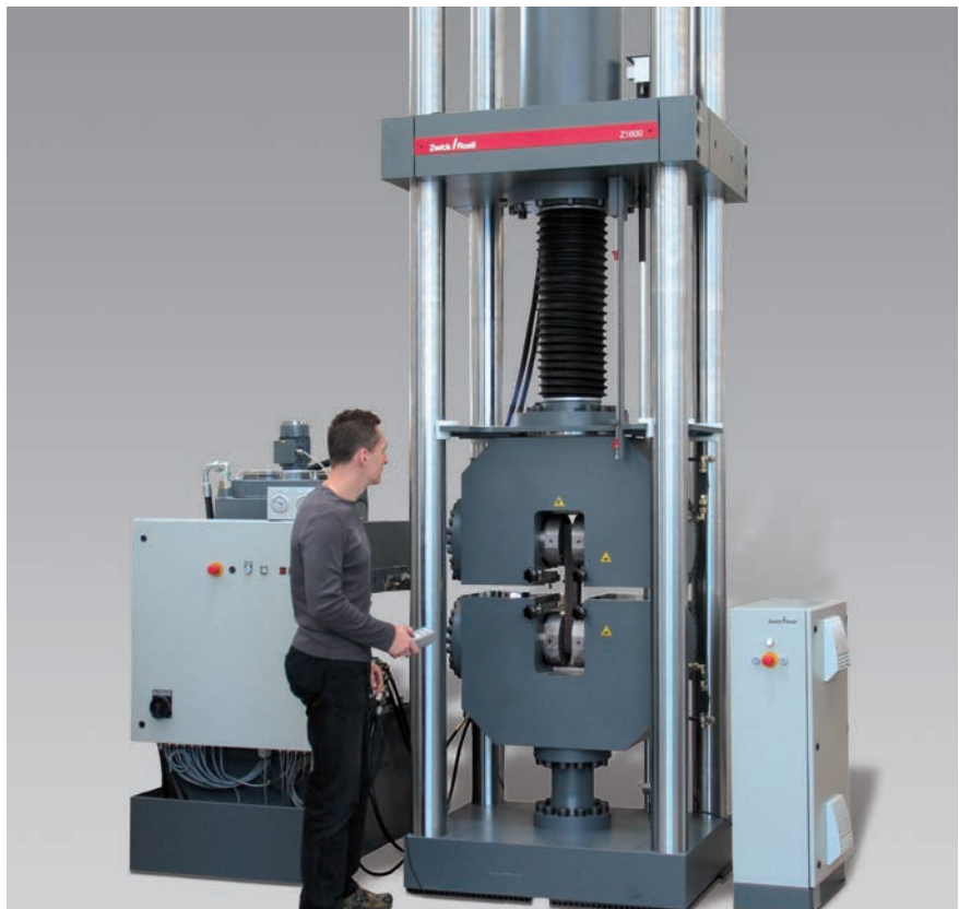
Fig.2: High-capacity testing machine with double-actuator hydraulic grips
