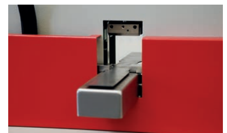
Fig.5: Measuring cross-section of a flat specimen
