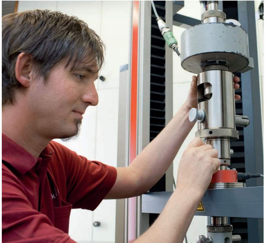
Fig.2: Every load cell undergoes a ZwickRoell factory calibration as soon as it enters service on a testing machine
