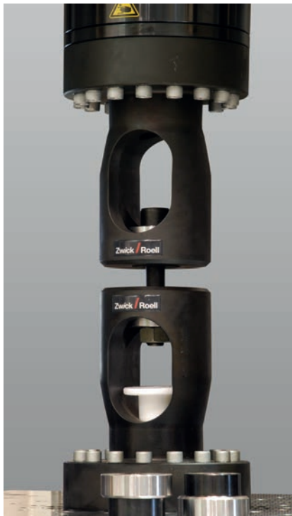
Fig.1: Fatigue test on threaded fasteners
