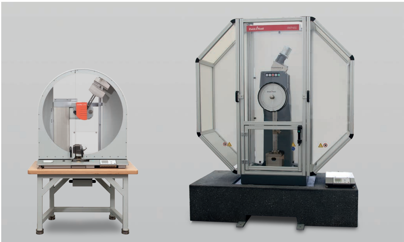
Fig.1: HIT 50P and RKP 450 pendulum impact testers for Charpy and Izod tests
