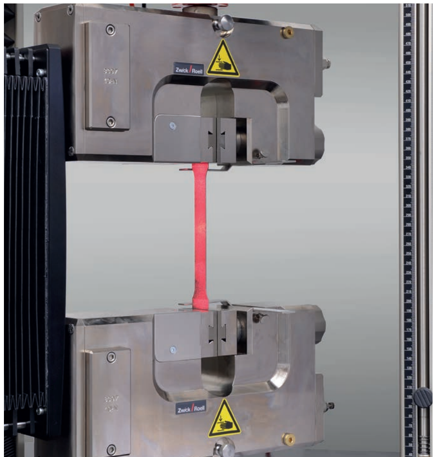
Fig. 1: Tensile test on thin sheet specimens with laserXtens Array extensometer
