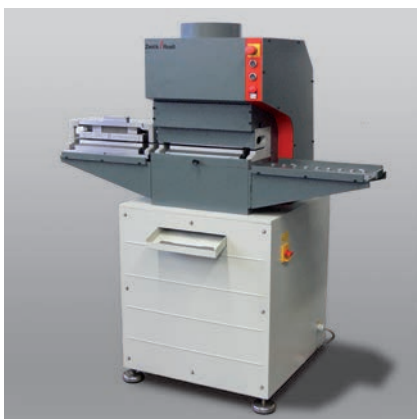
Fig.1: M-Cut 65 specimen blanking machine
