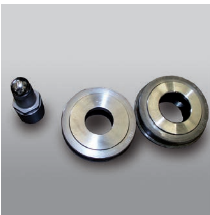
Fig.1: Cupping tool for Erichsen test
