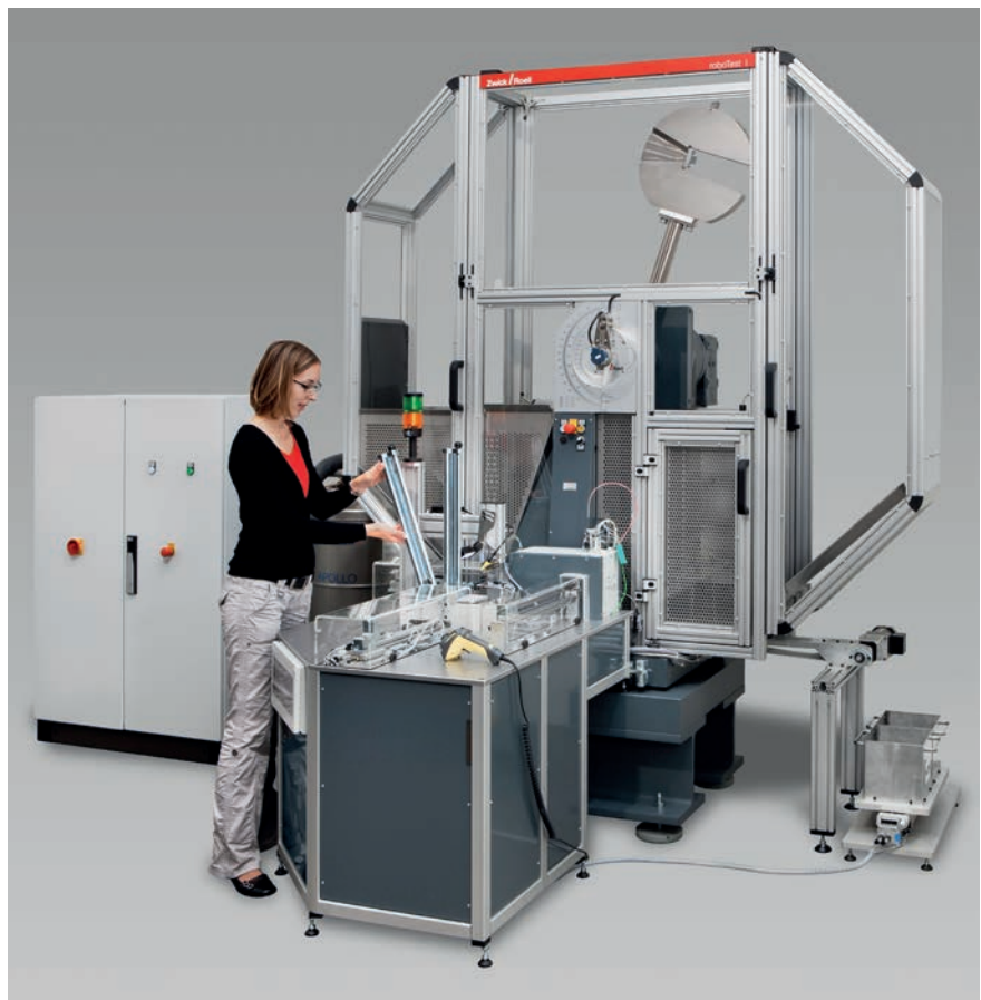
Fig. 2: roboTest I for automated Charpy and Izod tests (including specimen cooling)
