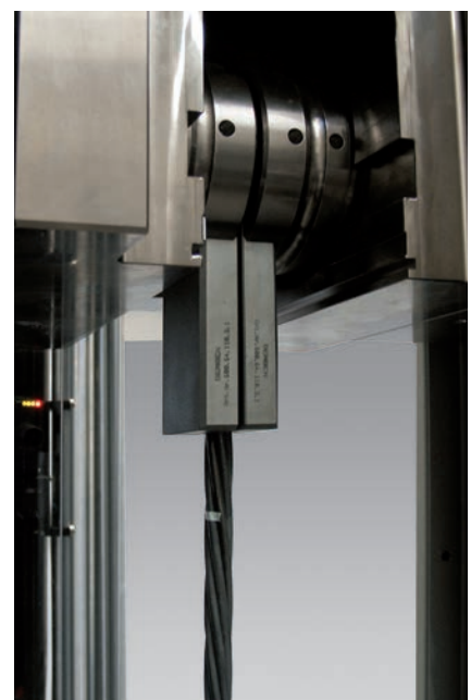
Fig.2: Clamping device for steel strand
