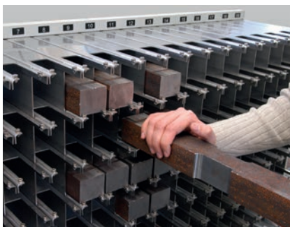
Fig. 2: roboTest P for automated tensile tests on heavy specimens, with additional sensors and measuring devices incorporated e.g. cross-section measuring device, bottom right)
