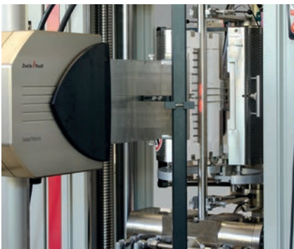
Fig.1: High-temperature furnace with laserXtens
