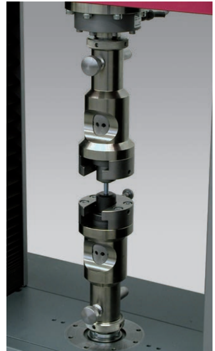
Fig.2: Tensile test on threaded fasteners
