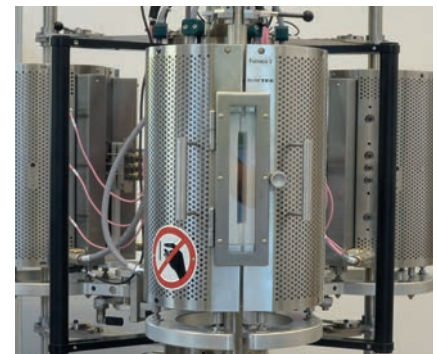
Fig.5: Carousel with 3 high-temperature furnaces
