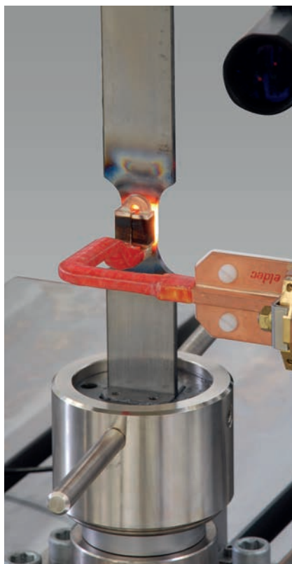
Fig.2: High-speed tensile test at high temperature
