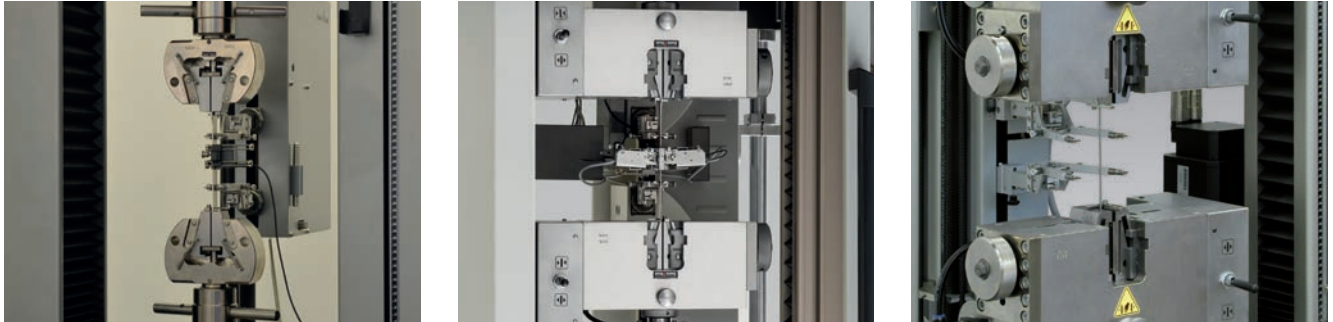
Fig.1: Wedge grips and wedge/wedge-screw grips
