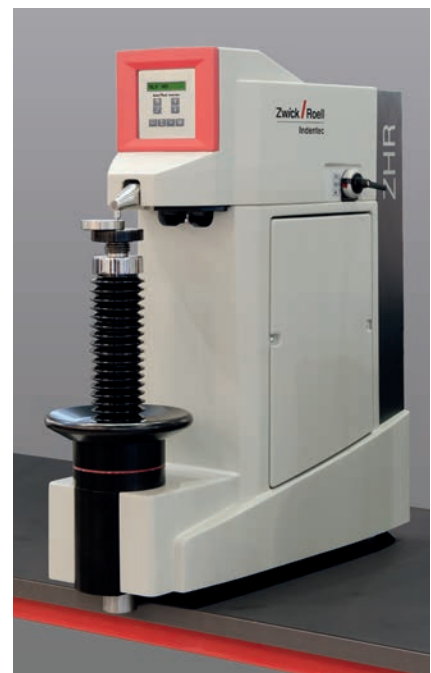
Fig.3: ZHR 4150 LK Rockwell hardness tester
