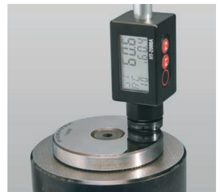
Fig.3: HT1000/2000 rebound hardness tester
