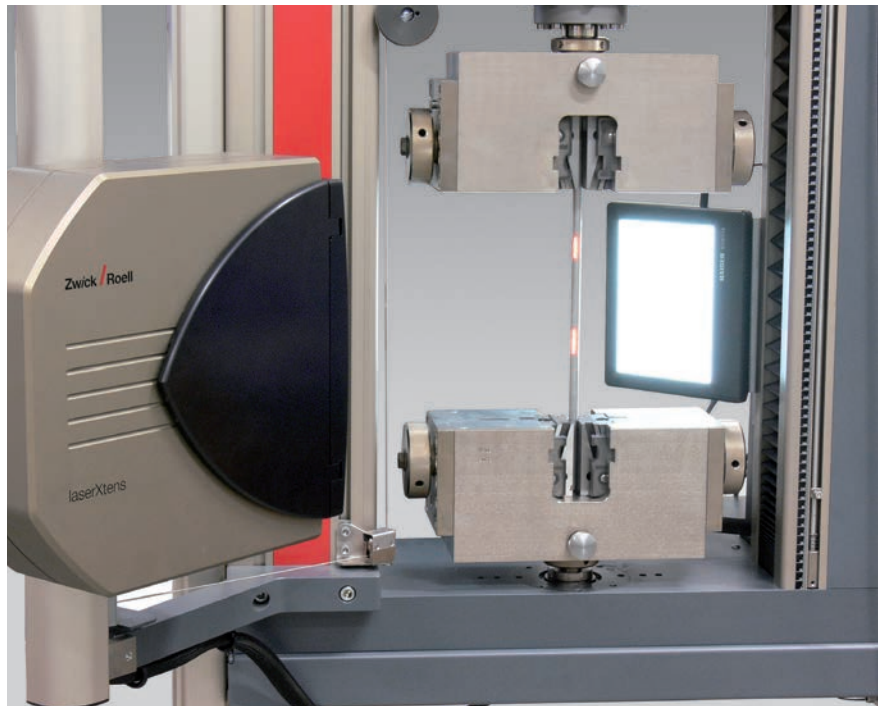
Fig.1: laserXtens extensometer with videoXtens option for transverse strain
