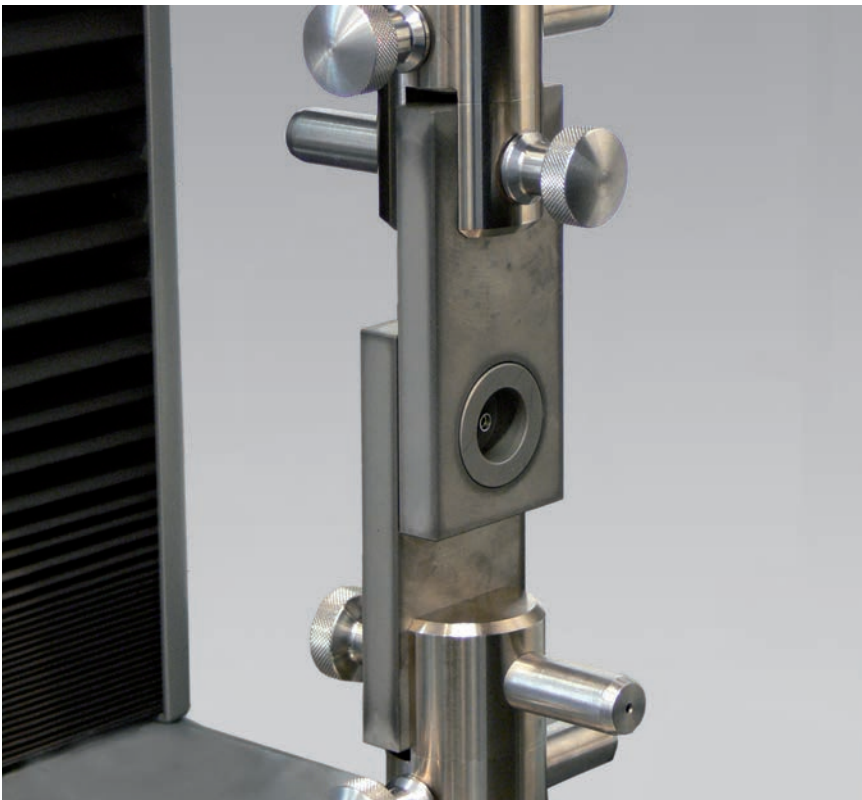
Fig.1: Shear test on riveted joint
