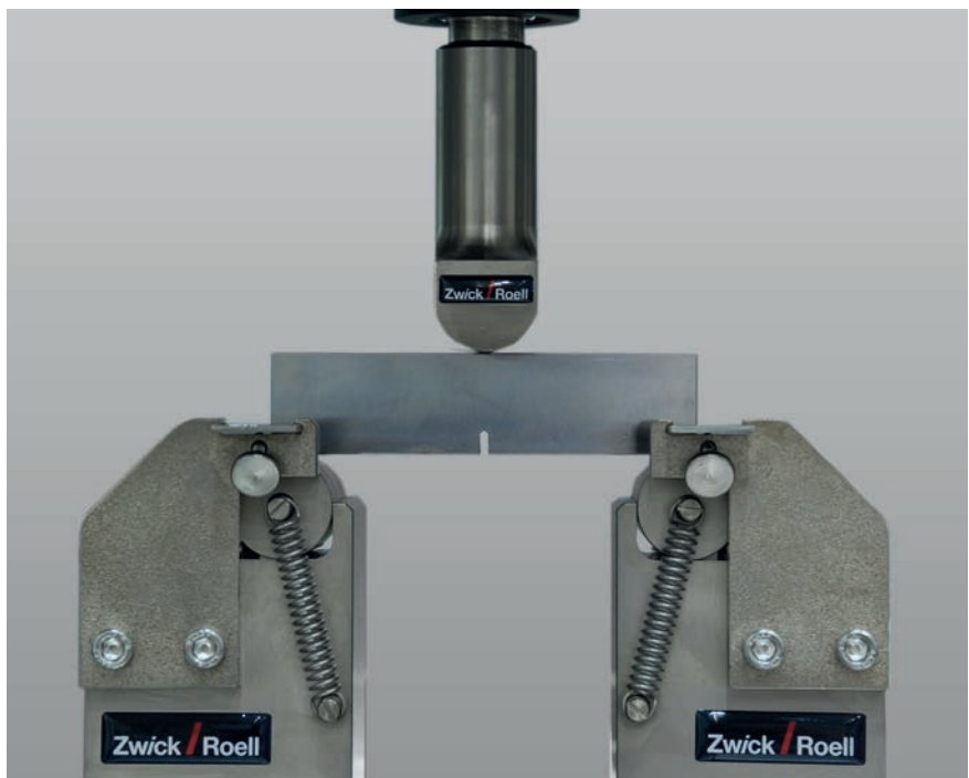
Fig.2: SENB specimen in Vibrophore
