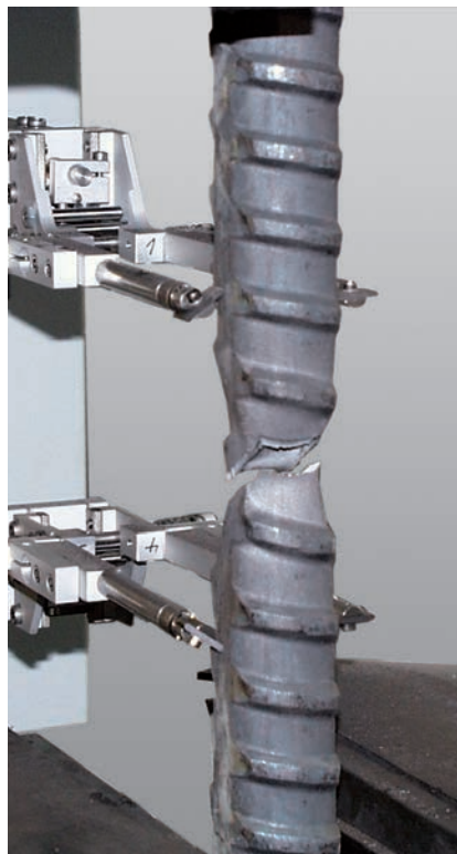
Fig.1: Tensile test on steel rebar with makroXtens extensometer
