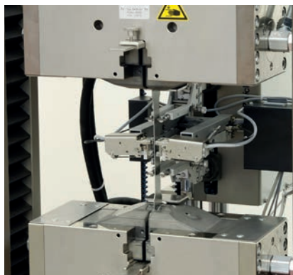
Fig. 1: makroXtens and variants with optional fine-strain measurement (bottom)
