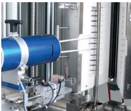
Fig.2: High-temperature furnace with HT extensometer
