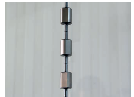
Fig.3: Testing for hydrogen embrittlement as per ASTM F519
