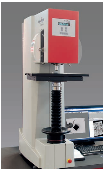
Fig.1: ZHU250CL universal hardness tester
