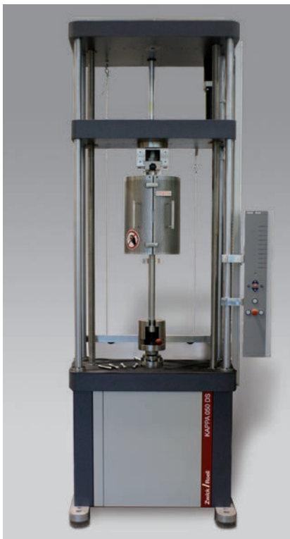
Fig.1: KAPPA DS (left) and KAPPA SS - CF (right) electromechanical creep testing machines
