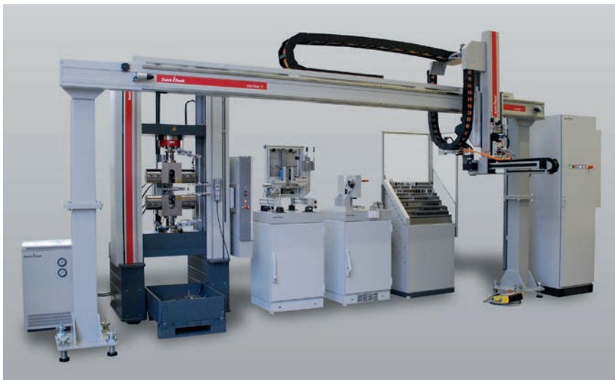
Fig. 1: roboTest R for automated tensile tests on sheet metals, rods and reinforcing steel
