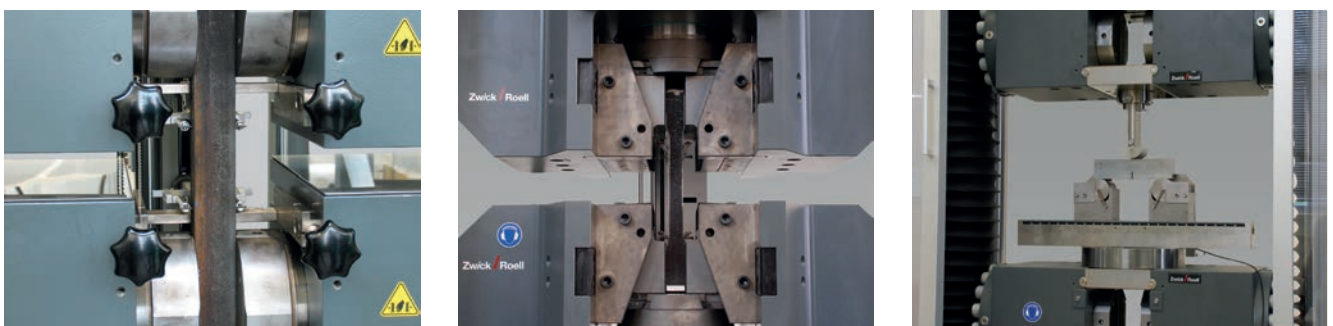
Fig.4: Heavy-duty hydraulic grips for testing applications up to 2,500 kN
