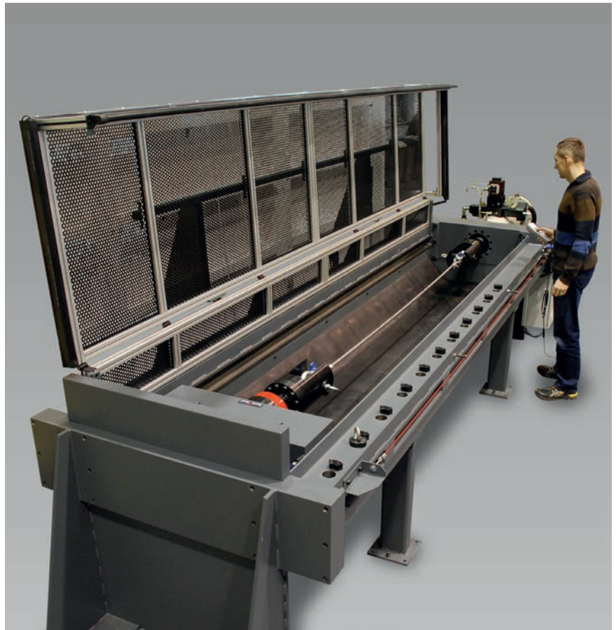
Fig.1: Servo-hydraulic horizontal testing machine for cyclic tests on wire ropes
