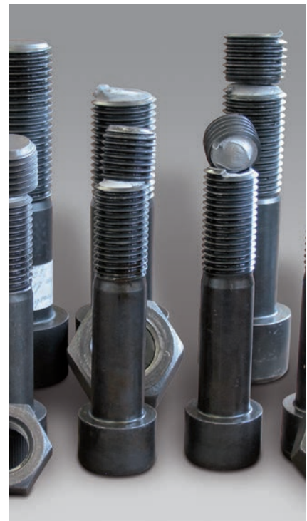
Fig.3: Bolts after testing
