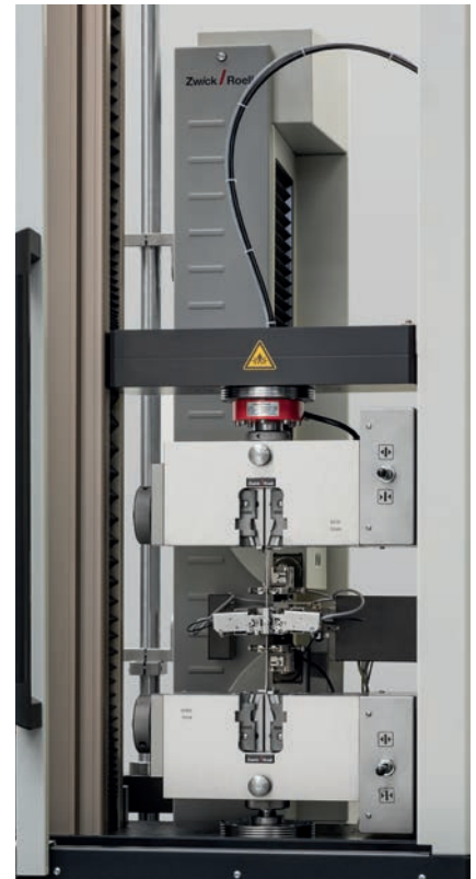
Fig. 4: multiXtens with optional fine-strain and transverse-strain measurement
