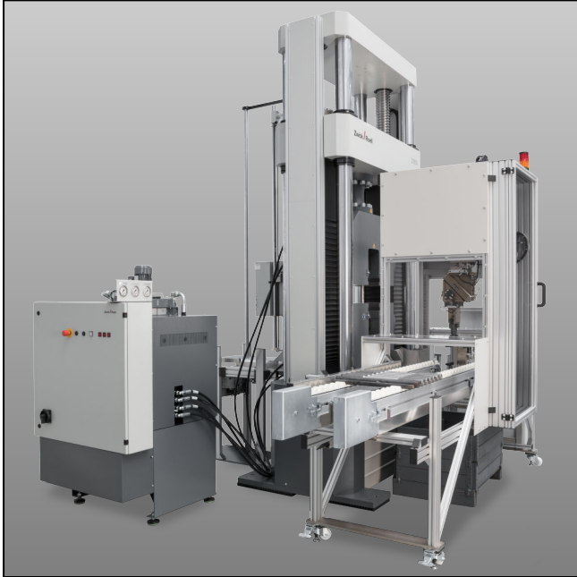
'roboTest C' robotic testing system
