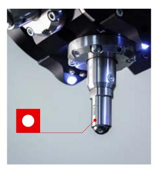
It is important to note that Brinell hardness testing may not be suitable for materials with very high hardness or thin and small components where a smaller indentation size is desired. In such cases, alternative hardness testing methods like Knoop or Vickers may be more appropriate.
