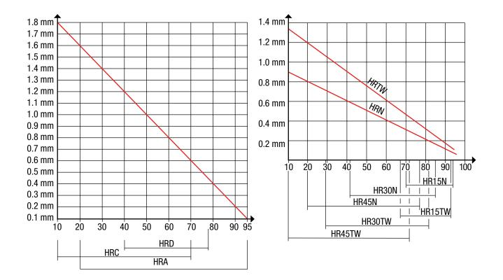
Minimum thickness (hardness coat) of the sample in relation to Rockwell hardness
