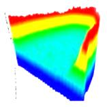
• Up to 10000 test points: hardness mapping refers to the creation of a comprehensive hardness curve for a specimen or a specific area. The hardness curve can be determined through the equal distribution of test points across the entire specimen. The result – the hardness map – can either be shown as a 2D color image or a 3D diagram.
